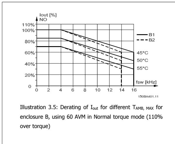
Illustration 3.5: Derating of  $I_{out}$  for different  $T_{AMB, MAX}$  for enclosure B, using 60 AVM in Normal torque mode (110% over torque)
