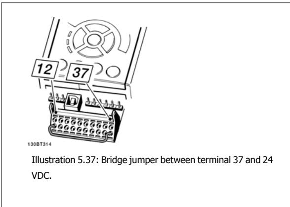
Illustration 5.37: Bridge jumper between terminal 37 and 24 VDC.
