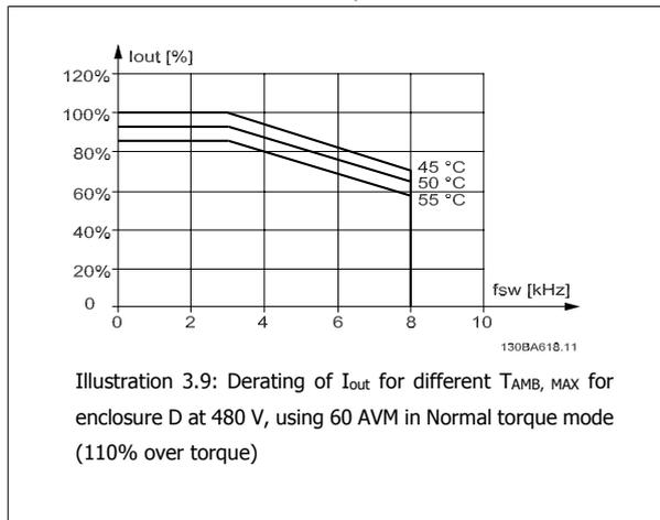
Illustration 3.9: Derating of  $I_{out}$  for different  $T_{AMB, MAX}$  for enclosure D at 480 V, using 60 AVM in Normal torque mode (110% over torque)
