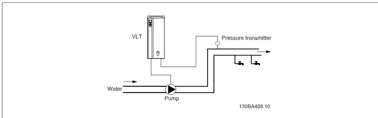
In a water distribution system, the pressure is to be maintained at a constant value. The desired pressure (setpoint) is set between 0 and 10 Bar using a 0-10 volt potentiometer or can be set by a parameter. The pressure sensor has a range of 0 to 10 Bar and uses a two-wire transmitter to provide a 4-20 mA signal. The output frequency range of the drive is 10 to 50 Hz.
