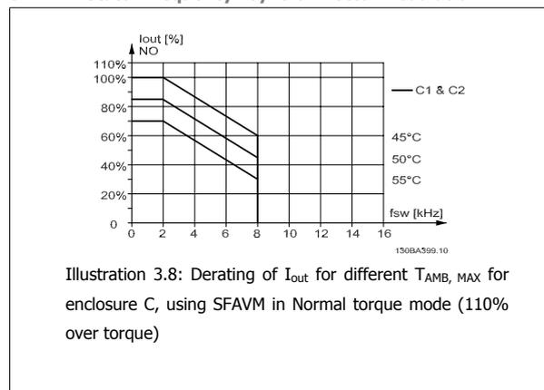
Illustration 3.8: Derating of  $I_{out}$  for different  $T_{AMB, MAX}$  for enclosure C, using SFAVM in Normal torque mode (110% over torque)
