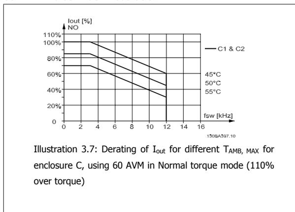
Illustration 3.7: Derating of  $I_{out}$  for different  $T_{AMB, MAX}$  for enclosure C, using 60 AVM in Normal torque mode (110% over torque)
