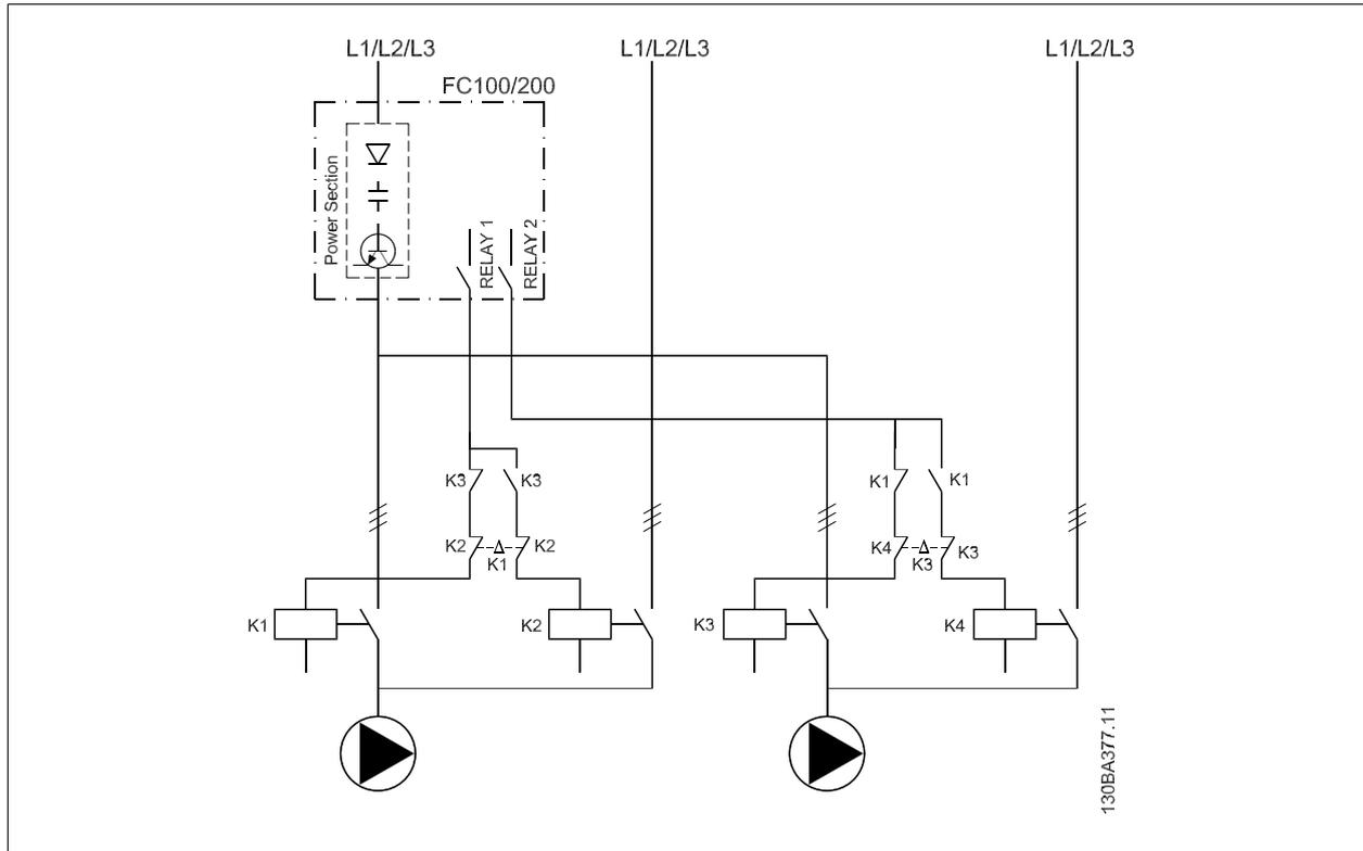
Every pump must be connected to two contactors (K1/K2 and K3/K4) with a mechanical interlock. Thermal relays or other motor protection devices must be applied according to local regulation and/or individual demands.
