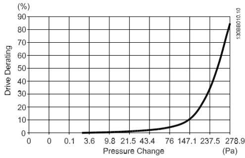
Illustration 3.31: E Frame Derating vs. Pressure Change (Small Fan), P250T5 and P355T7-P400T7
