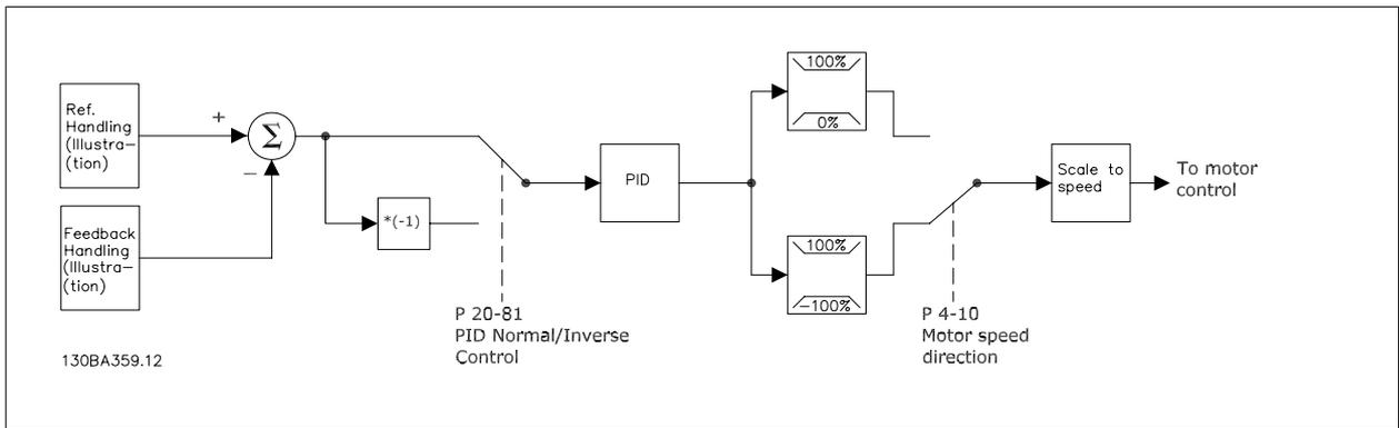
**NB!** While the default values for the drive's Closed Loop controller will often provide satisfactory performance, the control of the system can often be optimized by adjusting some of the Closed Loop controller's parameters. It is also possible to autotune the PI constants.
