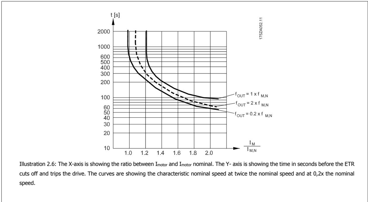
Illustration 2.6: The X-axis is showing the ratio between  $I_{motor}$  and  $I_{motor}$  nominal. The Y- axis is showing the time in seconds before the ETR cuts off and trips the drive. The curves are showing the characteristic nominal speed at twice the nominal speed and at 0,2x the nominal speed.
