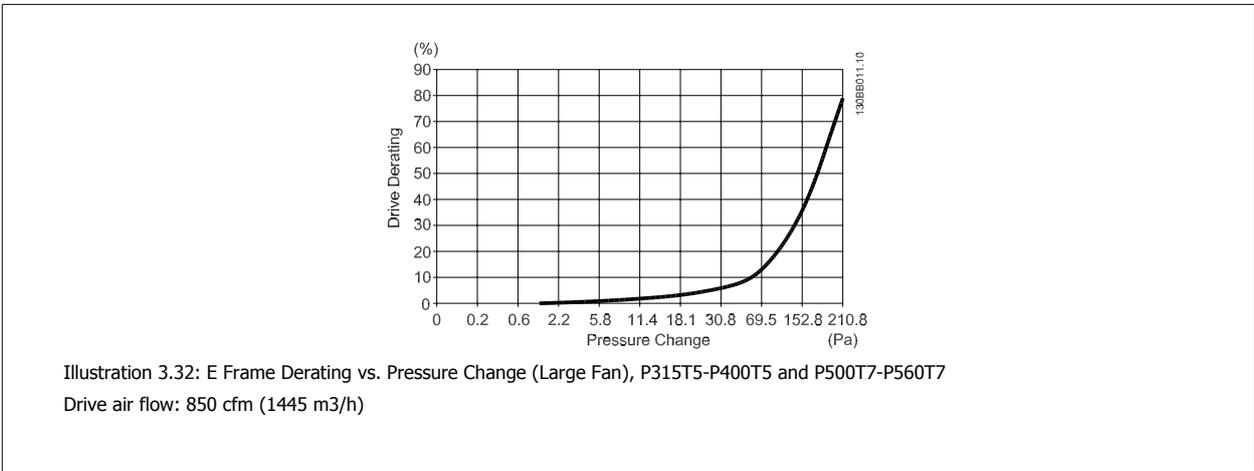
Illustration 3.32: E Frame Derating vs. Pressure Change (Large Fan), P315T5-P400T5 and P500T7-P560T7
