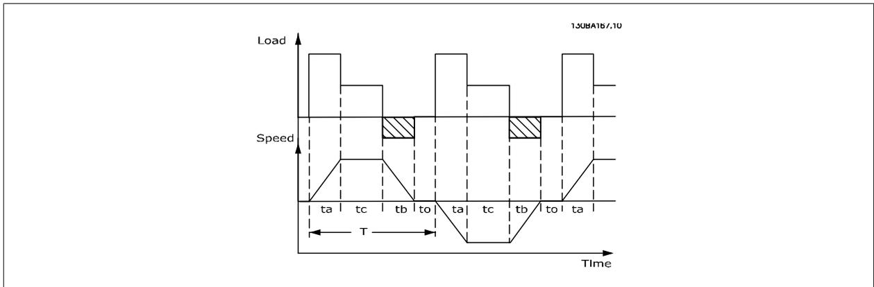
Danfoss offers brake resistors with duty cycle of 5%, 10% and 40% suitable for use with the FC202 AQUA drive series. If a 10% duty cycle resistor is applied, this is able of absorbing braking power upto 10% of the cycle time with the remaining 90% being used to dissipate heat from the resistor.
