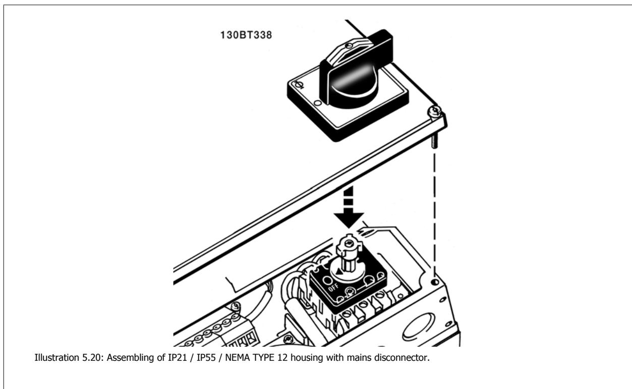
Illustration 5.20: Assembling of IP21 / IP55 / NEMA TYPE 12 housing with mains disconnect.
