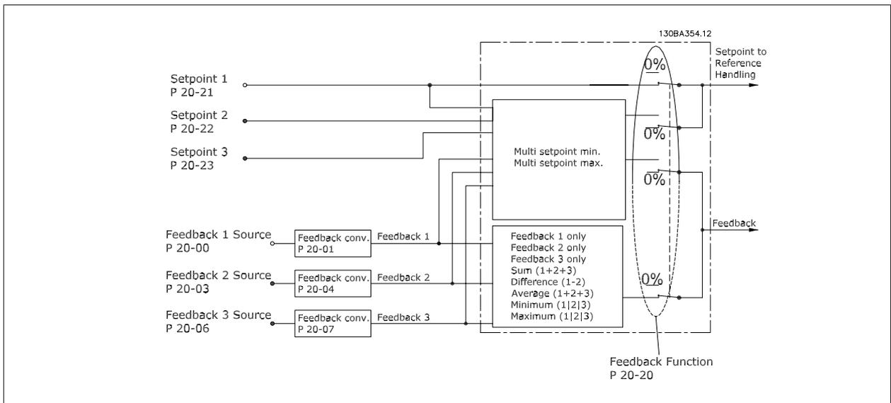
Feedback handling can be configured to work with applications requiring advanced control, such as multiple setpoints and multiple feedbacks. Three types of control are common.
