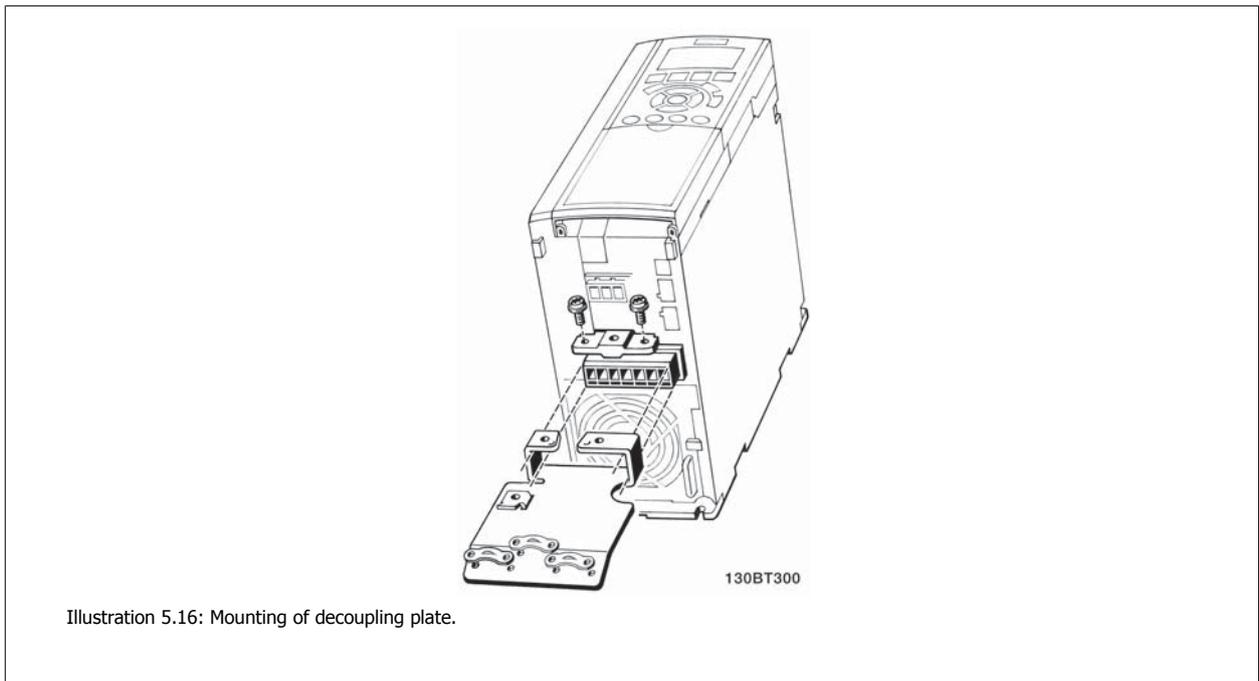
1. Fasten decoupling plate to the bottom of the frequency converter with screws and washers from the accessory bag.
