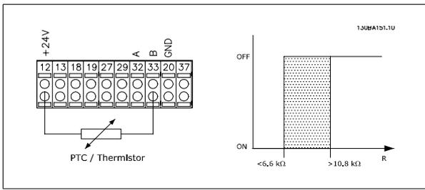
Using a digital input and 10 V as power supply:
