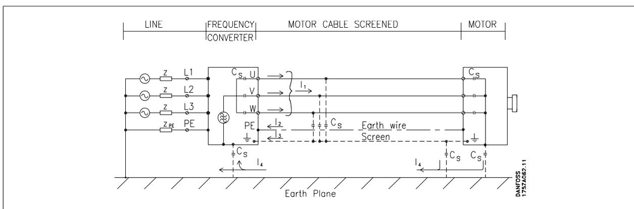
If the screen is to be placed on a mounting plate for the frequency converter, the mounting plate must be made of metal, because the screen currents have to be conveyed back to the unit. Moreover, ensure good electrical contact from the mounting plate through the mounting screws to the frequency converter chassis.
