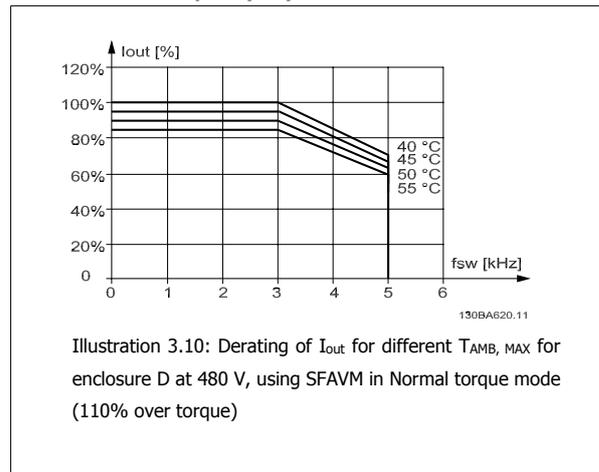
Illustration 3.10: Derating of  $I_{out}$  for different  $T_{AMB, MAX}$  for enclosure D at 480 V, using SFAVM in Normal torque mode (110% over torque)
