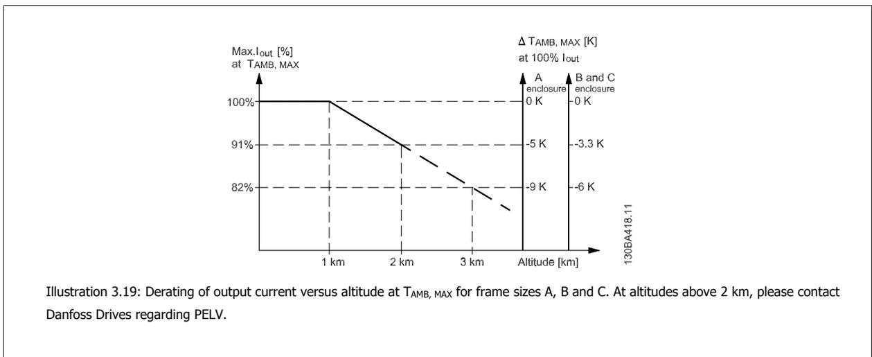
An alternative is to lower the ambient temperature at high altitudes and thereby ensure 100% output current at high altitudes. As an example of how to read the graph, the situation at 2 km is elaborated. At a temperature of 45° C ( $T_{AMB, MAX} - 3.3$  K), 91% of the rated output current is available. At a temperature of 41.7° C, 100% of the rated output current is available.
