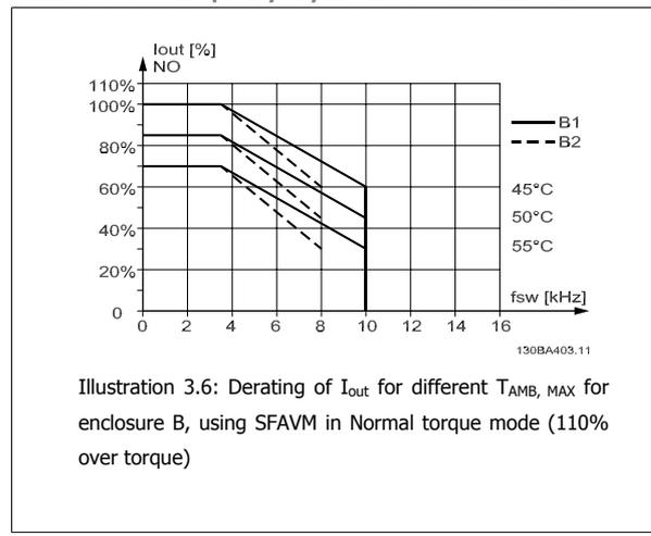
Illustration 3.6: Derating of  $I_{out}$  for different  $T_{AMB, MAX}$  for enclosure B, using SFAVM in Normal torque mode (110% over torque)
