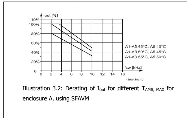
In enclosure A, the length of the motor cable has a relatively high impact on the recommended derating. Therefore, the recommended derating for an application with max. 10 m motor cable is also shown.
